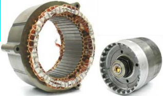
Powersplit Transmission: Planetary Gearset & 2 E-Machines
